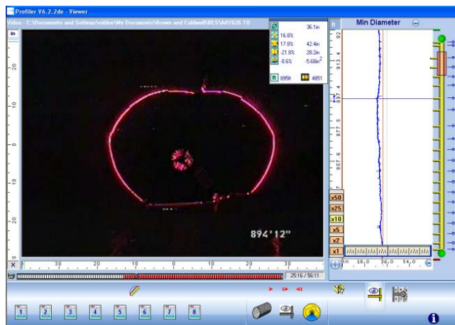
Figure G-12. Laser projection from laser profile inspection
